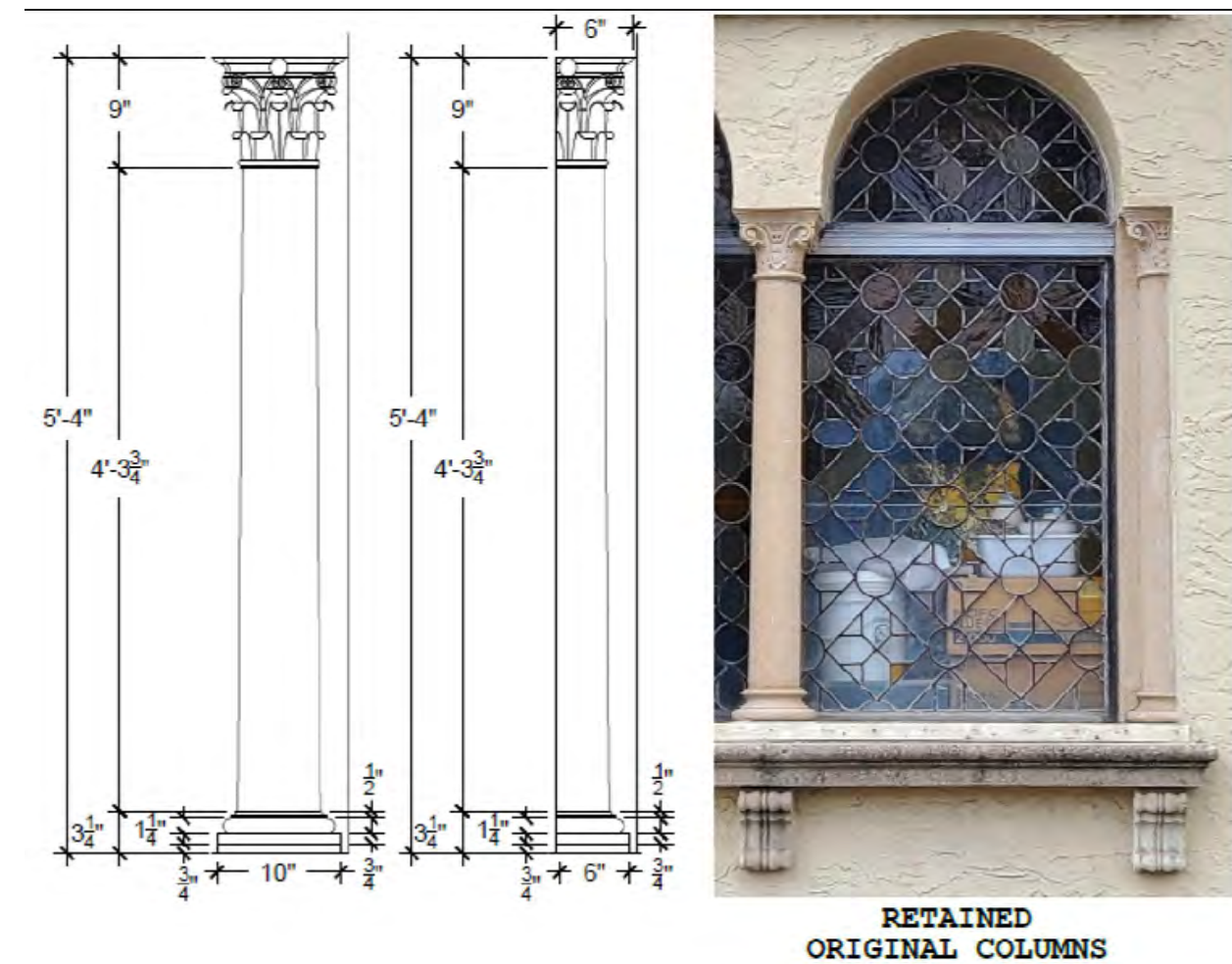
RETAINED ORIGINAL COLUMNS
