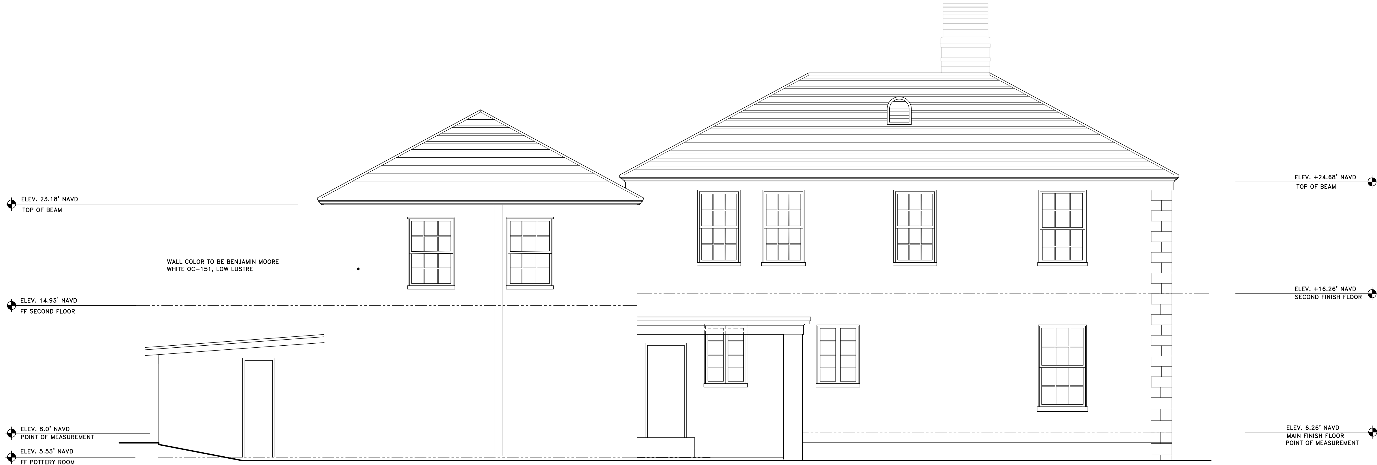
PROPOSED WEST ELEVATION SCALE: 1/4" = 1'-0" NO CHANGE, EXCEPT PAINT COLOR
