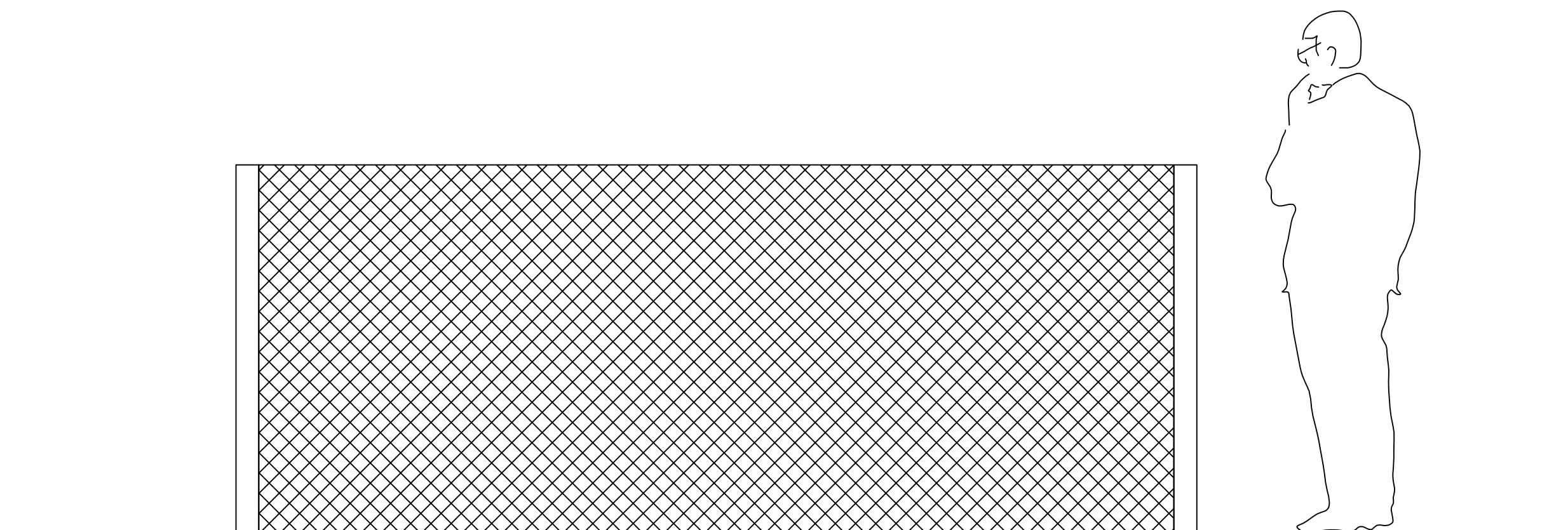
CHAIN LINK FENCE SCALE - 3/4"= 1'-0"
