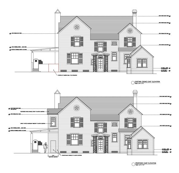
The addition is designed with a south-facing gable end. It will match the existing cedar shake shingle siding and wood shingle roof used in the 'Vicarage'. The design also features two (2) new impact-rated mahogany windows with a 6/1 divided-light pattern on the south and east facades. On
