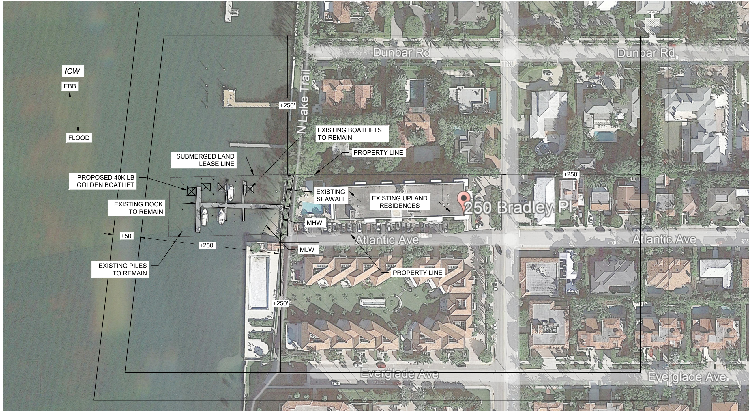
PROPOSED OVERALL BOATLIFT LAYOUT PLAN SCALE: 1" = 100'
