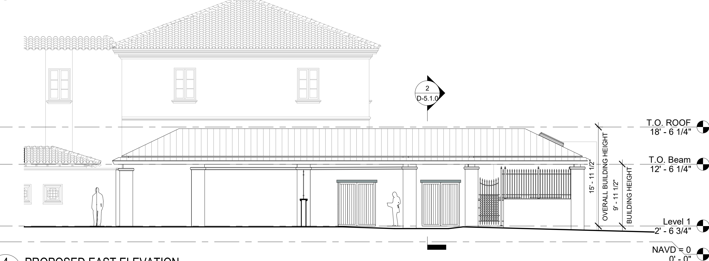
4 PROPOSED EAST ELEVATION D-4.1.0 1/8" = 1'-0"
