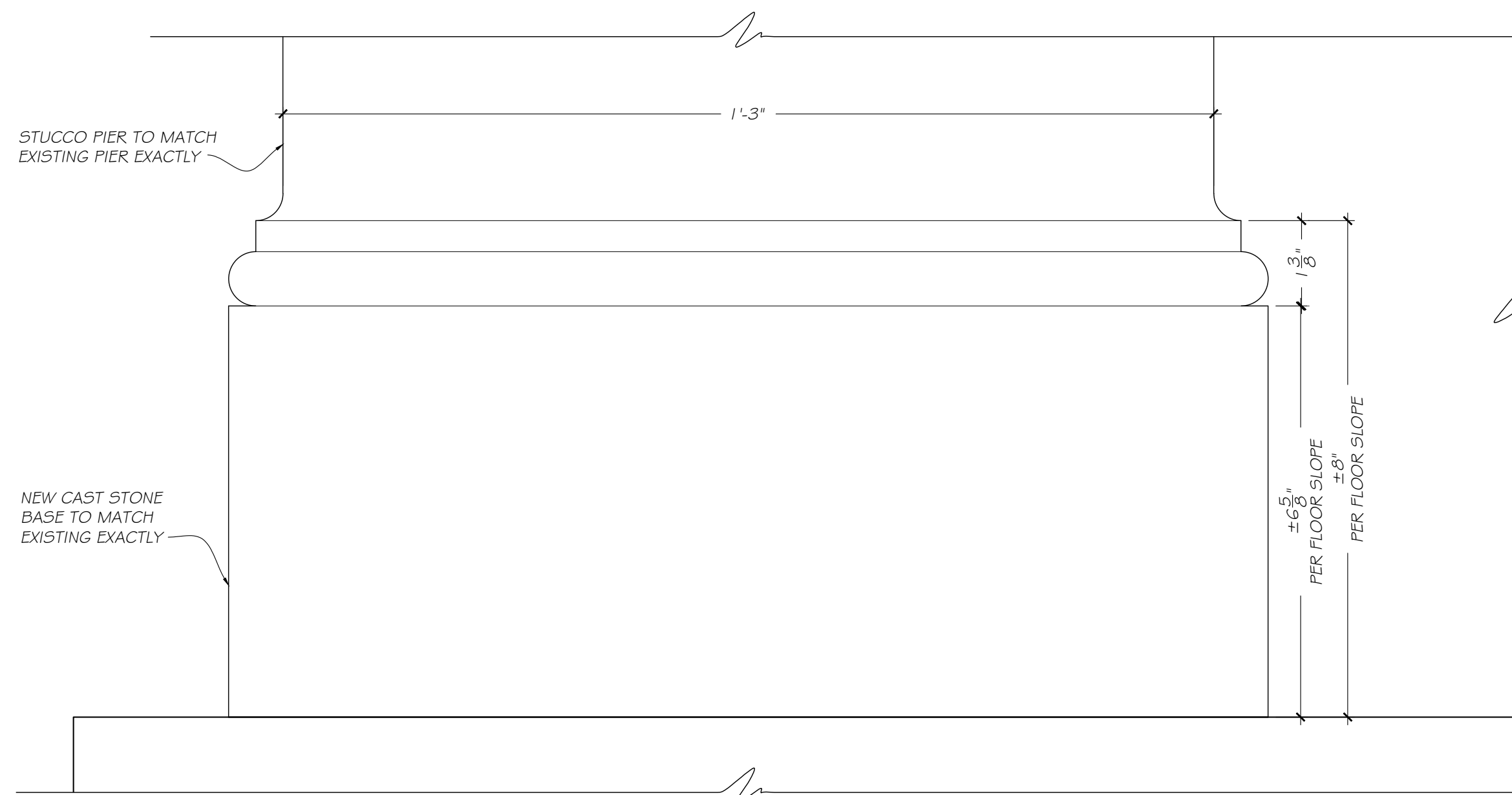
1 A-4.00C PROPOSED PIER BASE PROFILE 6" = 1'-0"
