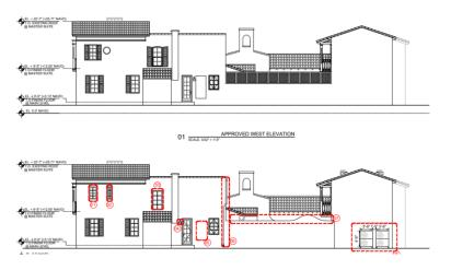
Additional changes are proposed interior to the courtyard which include adjustments to shutters, removal of shutters, revised railing designs, and redesign of the wall of the barbeque area.
