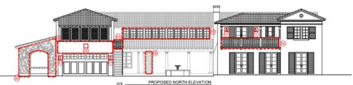
use of double nung windows is a better option for consistency with the original plans. The use of casement windows can be mitigated with divided-light patterns that replicate the appearance of sash windows with a wider (central) horizontal muntin.
