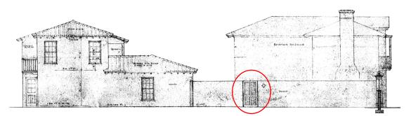
On the west side of the property, the site wall will be modified by removing the existing lattice and increasing the height with a curved design. In addition, ground-mounted mechanical equipment will be installed. These changes require variances, as discussed in the next section.
