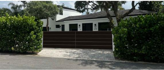
The proposed gate requires a variance as the required backup space is not being met, potentially creating an unsafe condition or blockage within the roadway. The applicant has provided 9'-5" of clearance where 18'-0" is needed. It is important to note that Via Marila is a very narrow roadway of only approximately 30'-0' wide.
