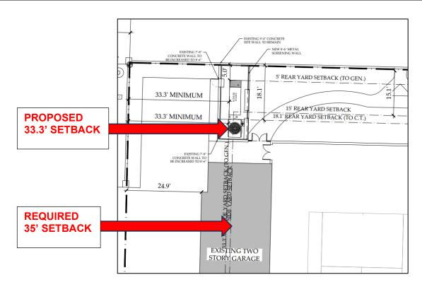
As the diagram below illustrates, **Variance 3** occurs because a higher enclosure wall height is needed to screen the replacement cooling tower and generator.
