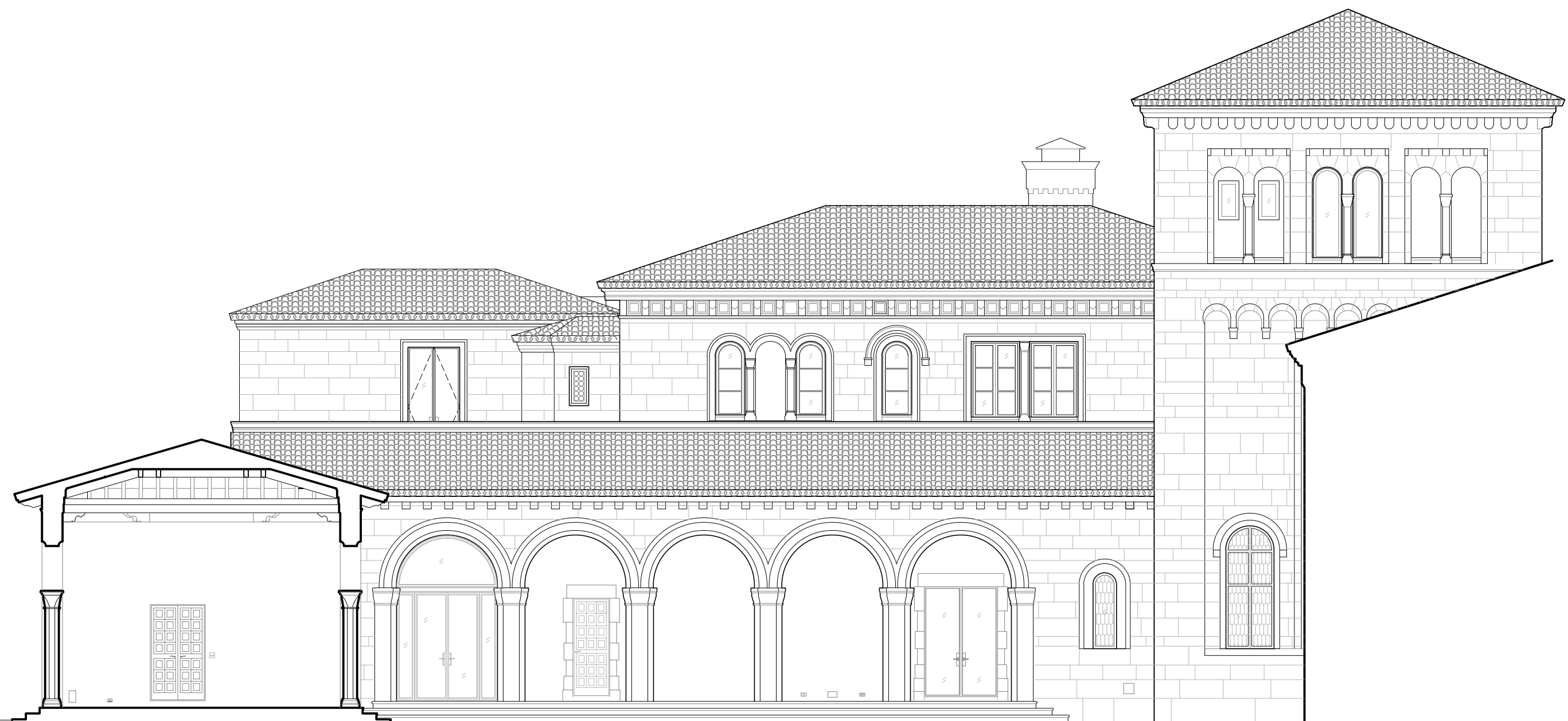
3 A247.0 PROPOSED WEST COURTYARD ELEVATION 1/8" = 1'-0"
