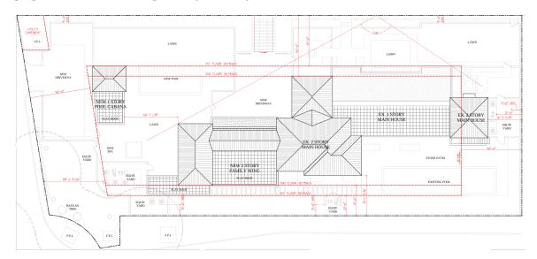
The residence's massing features one-story and two-story volumes. The two-story volumes and cabana structure feature hipped roofs with flat concrete tiles. The one-story portions are flat roofs with parapets. Exterior detailing includes metal banding details, stucco finish reveal, full view windows and doors to match existing, and glass balcony railings to match existing.
