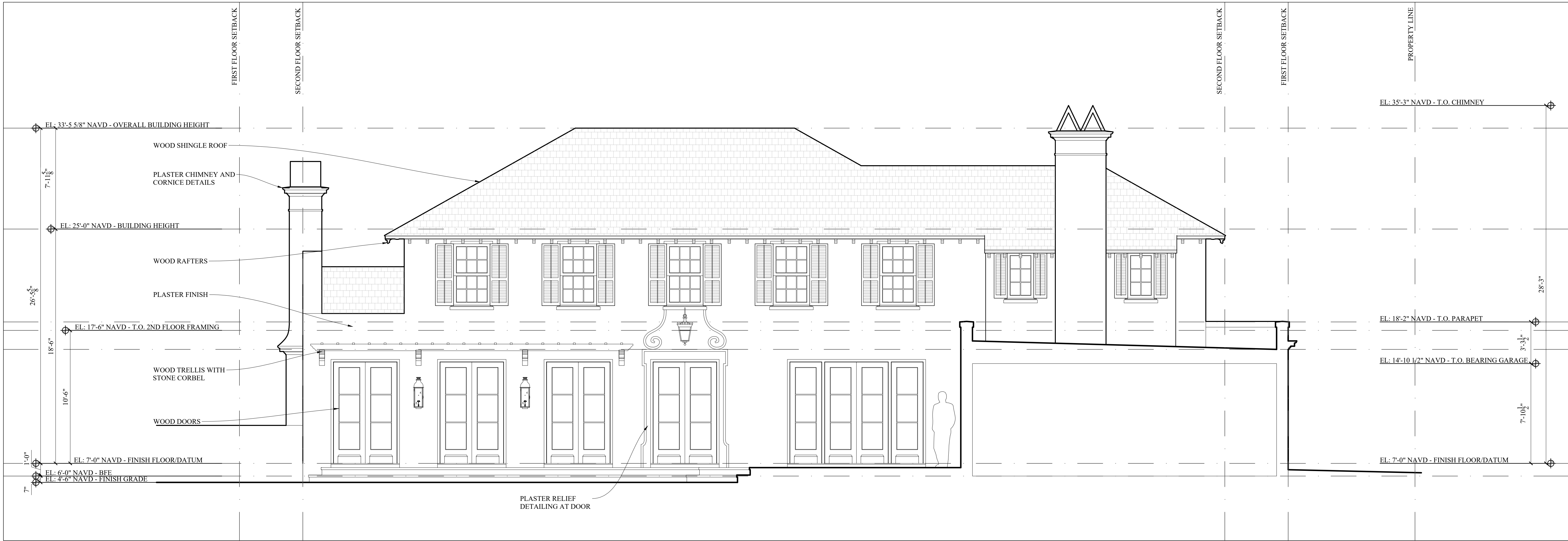
A SOUTH ELEVATION FROM INNER COURT SCALE: 1/4" = 1'-0"
