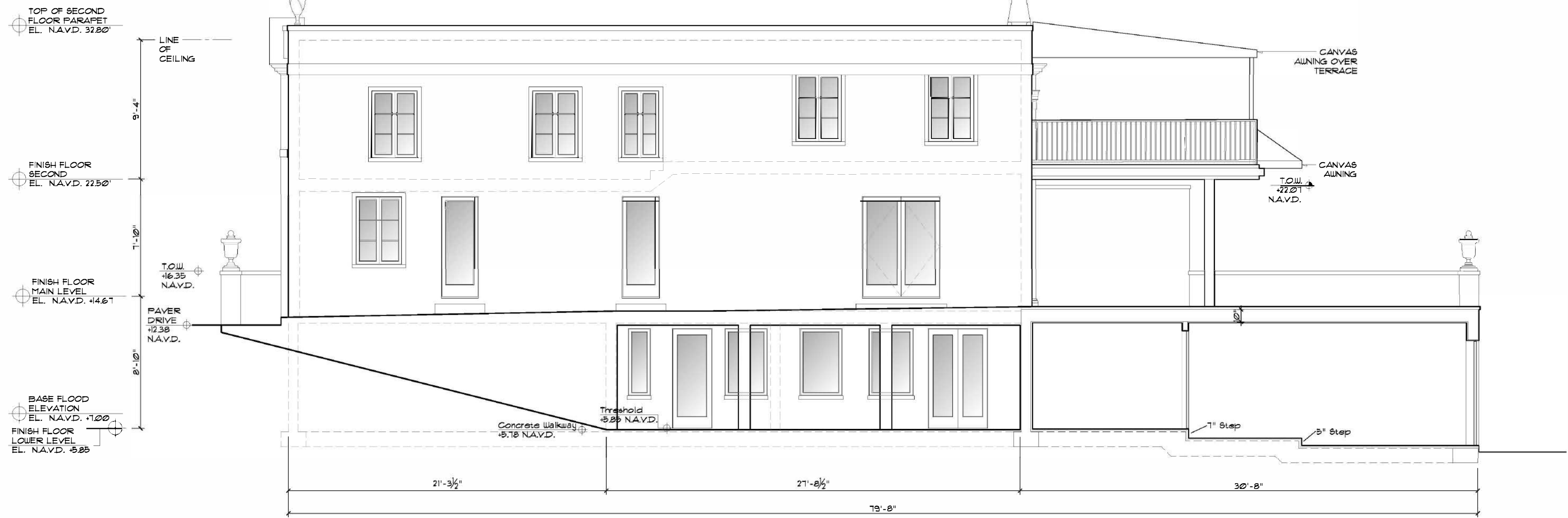
Existing North Elevation
