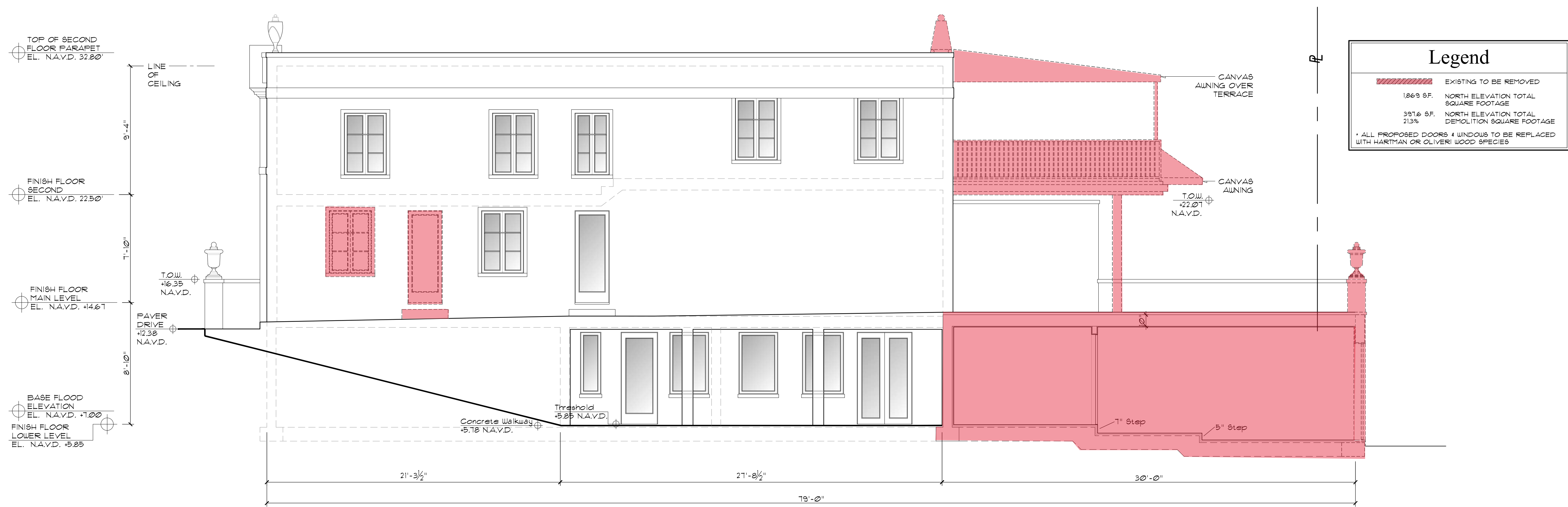
Demolition - North Elevation
