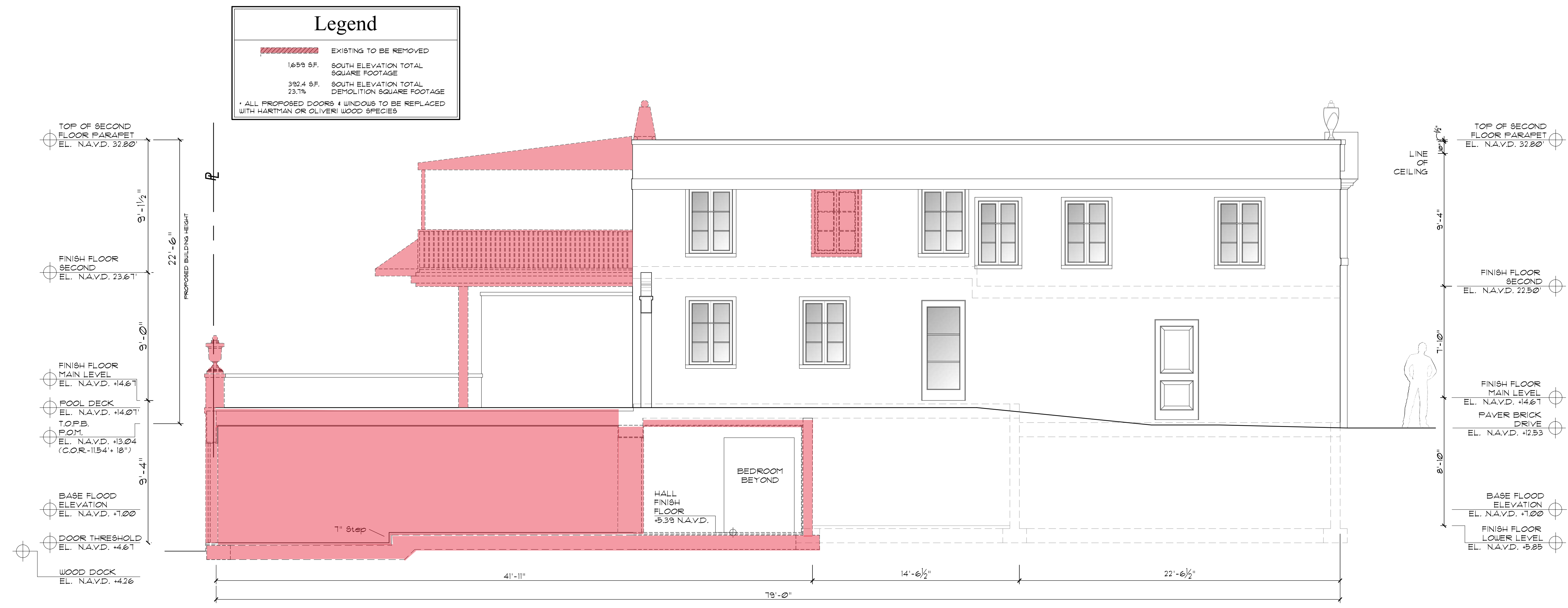
Demolition - South Elevation
