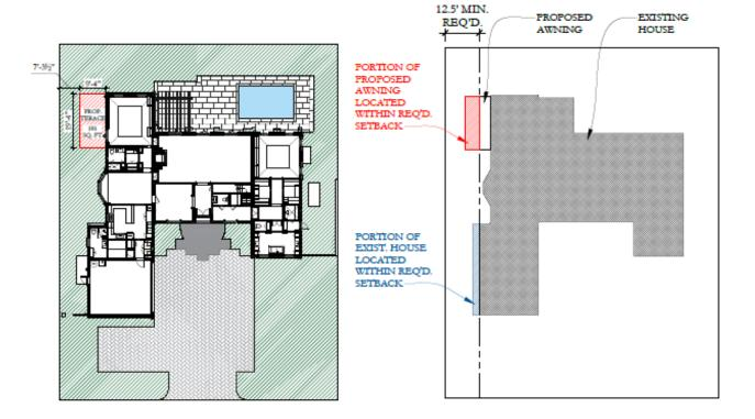
The proposed paving at the new proposed terrace is set to match existing paving material at the pool deck (seychelles limestone), cut in similar dimensions. As for the retractable awning, the setback dimension is calculated at its most extended configuration. The applicant has submitted
