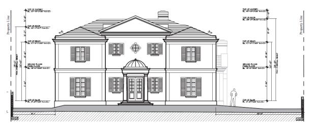
The applicant is proposing the construction of a new two-story residence. The proposed structure is neo-classical influenced style with smooth finish stucco painted a yellow color with white casement windows, doors, railings, shutters and trim. Roof material is proposed to be white flat
