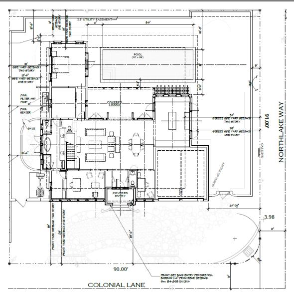
The proposed residence is designed with a Dutch-Caribbean influence including Dutch gable entry on the primary façade with cypress front doors, sidelights and fanlight transom, and gable ends at the two-story massing. Exterior building materials include white painted stucco walls, white concrete tile roof, copper gutters, painted aluminum Bahama shutters, and painted railings and trim.
