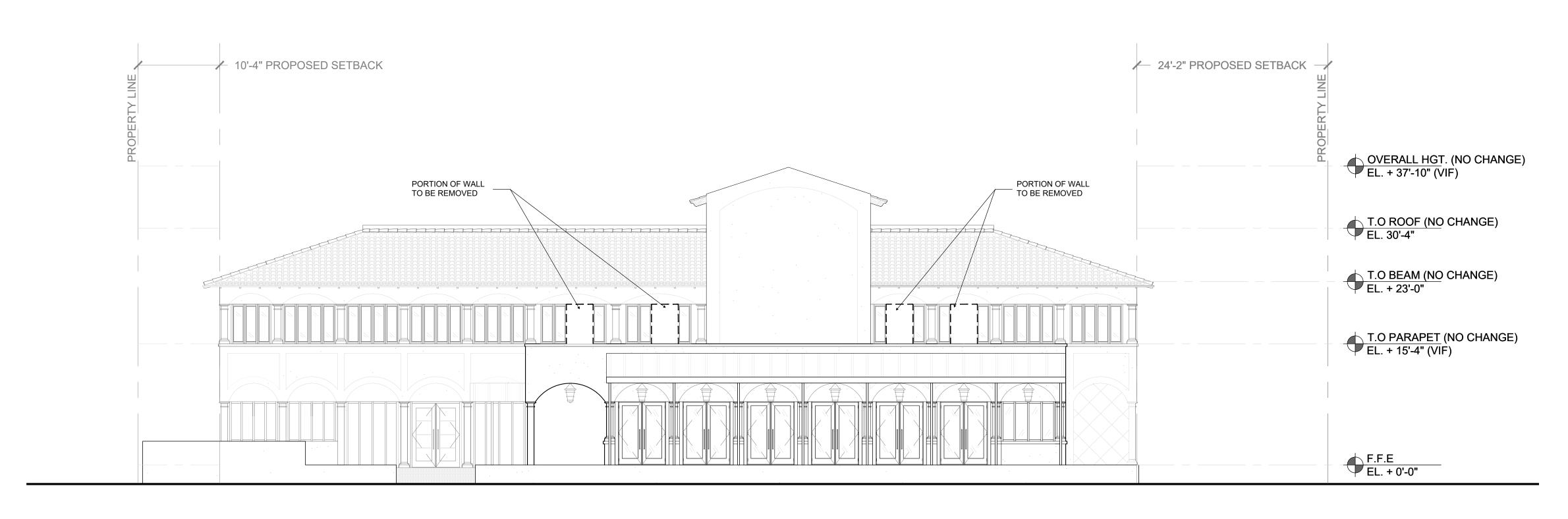
DEMOLITION SOUTH ELEVATION  $\frac{1}{\text{SCALE:} \frac{1}{8}" = 1'-0"}$
