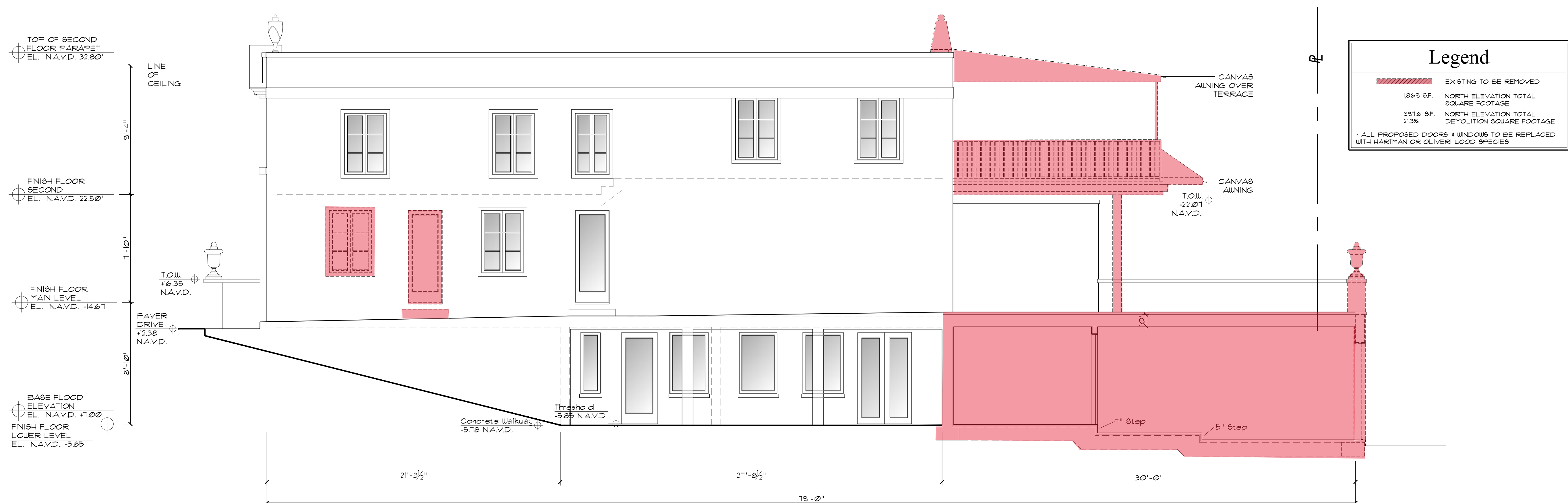
Demolition - North Elevation
