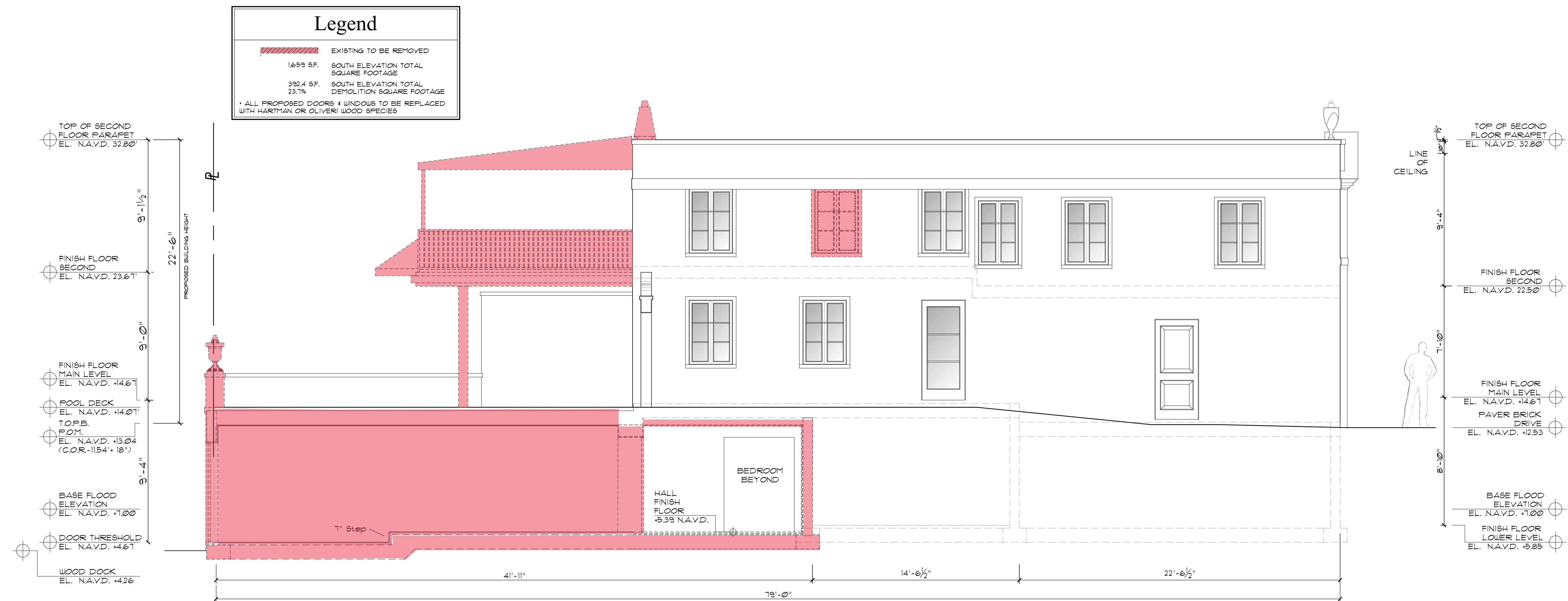
Demolition - South Elevation
