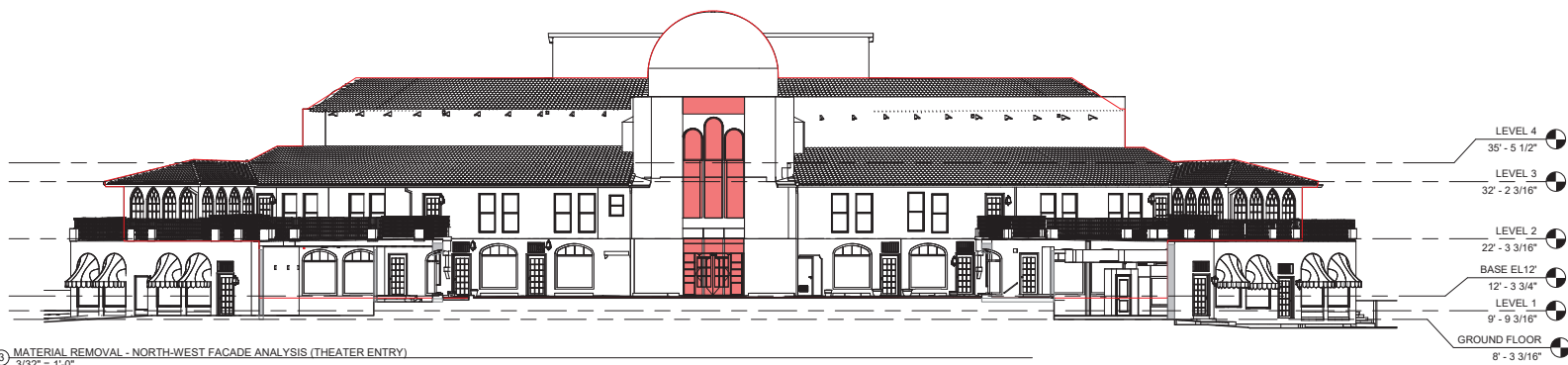
③ MATERIAL REMOVAL - NORTH-WEST FACADE ANALYSIS (THEATER ENTRY) 3/32" = 1'-0"
