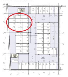
Kimley Horn and Associates, Inc.'s 04/18/23 Response: This condition was shown for only a total of four parking spaces and will only be used on infrequent occasions as it is anticipated that these would be the last parking spaces utilized only when other parking is full. Due to the minimal number and minimal usage of these spaces, it is anticipated that valet operators will be able to manage this parking during the few times in which they are in use.
