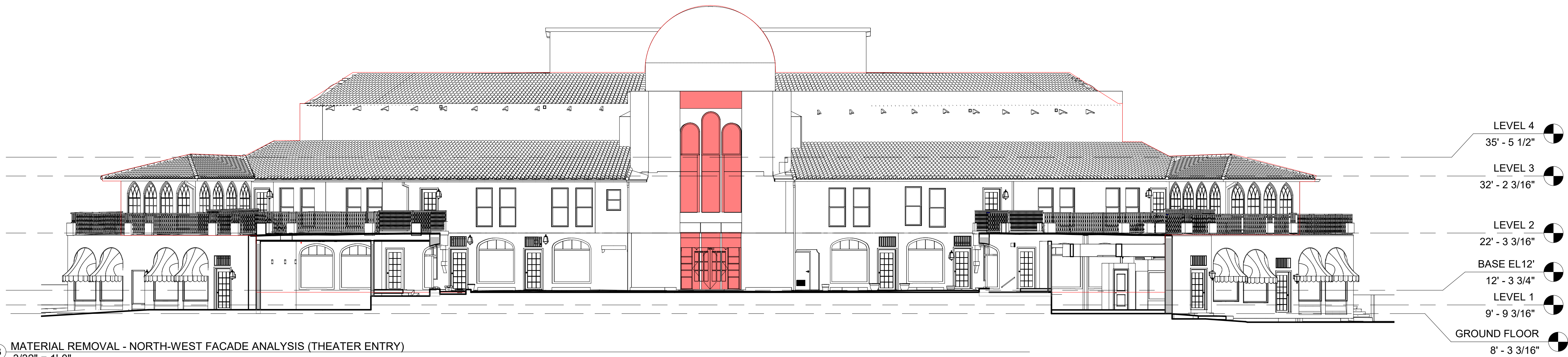
③ MATERIAL REMOVAL - NORTH-WEST FACADE ANALYSIS (THEATER ENTRY) 3/32" = 1'-0"
