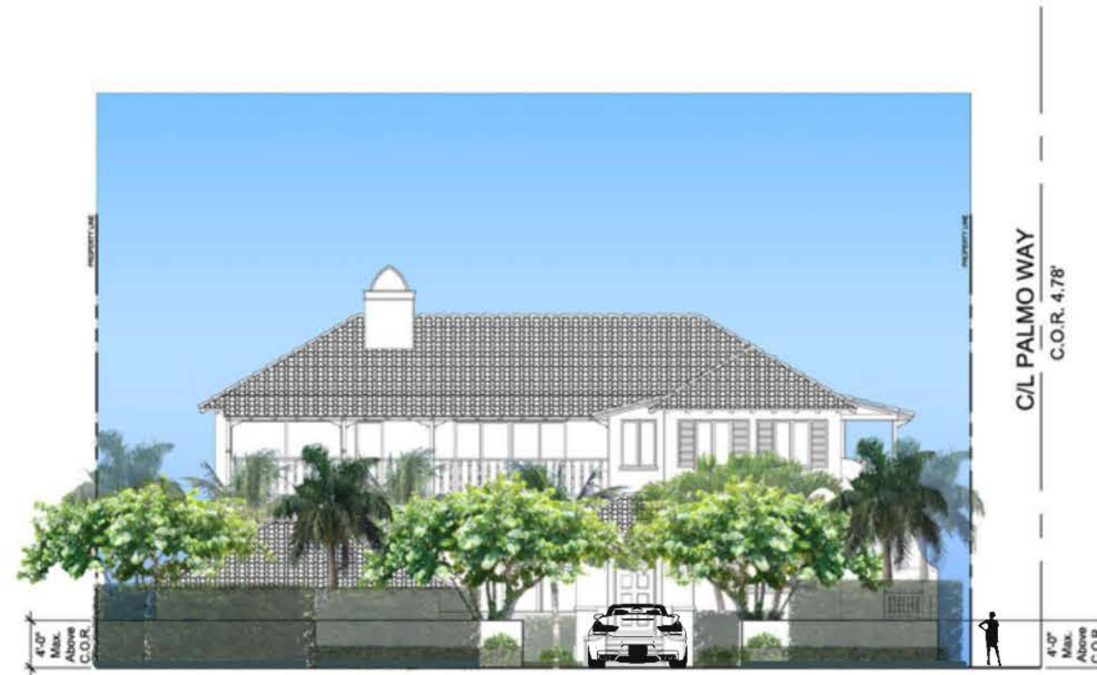
EXISTING EAST ELEVATION W/PROPOSED SITE WALL
