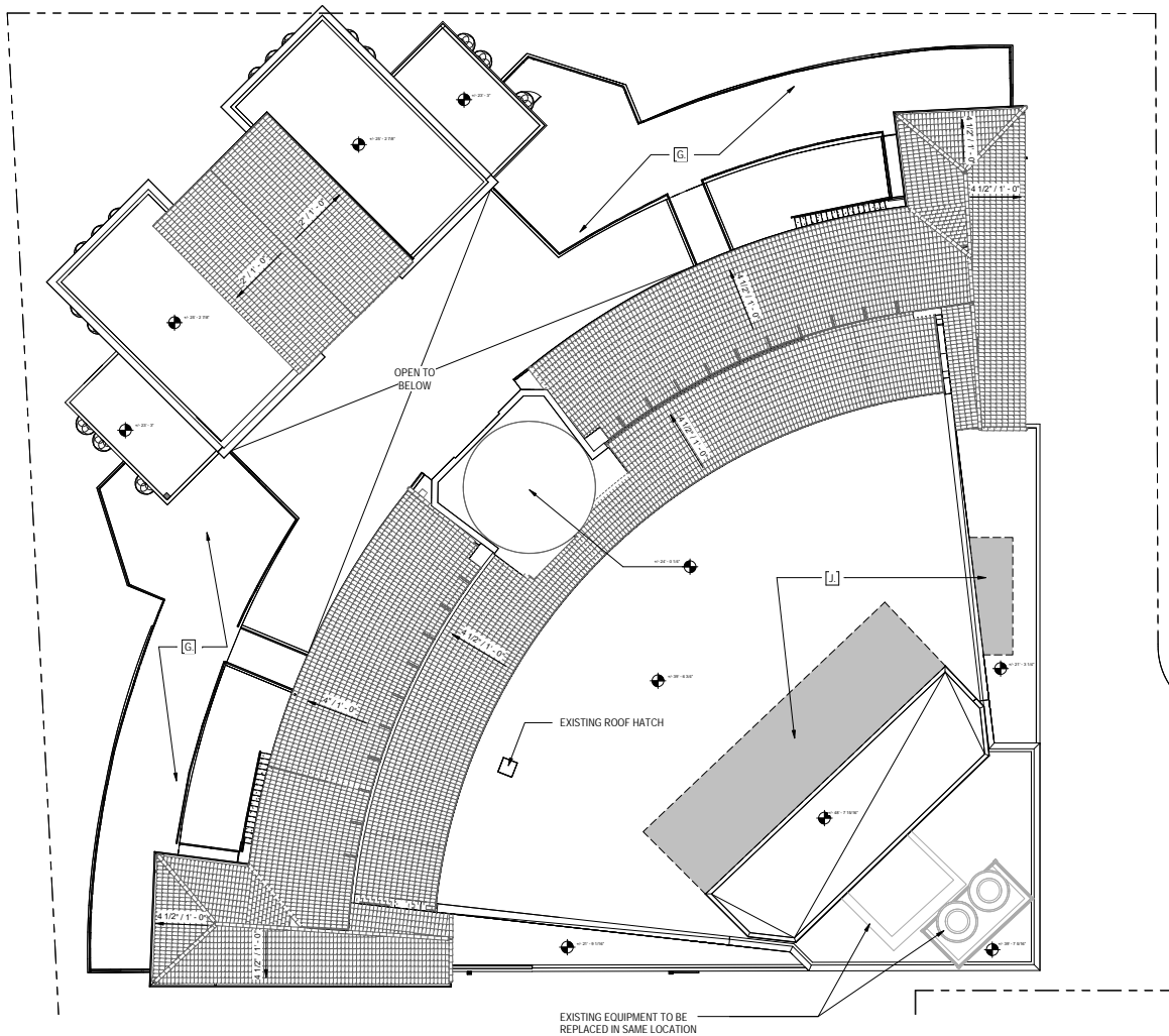
① MATERIAL REMOVAL PLAN - ROOF 3/32" = 1'-0"
