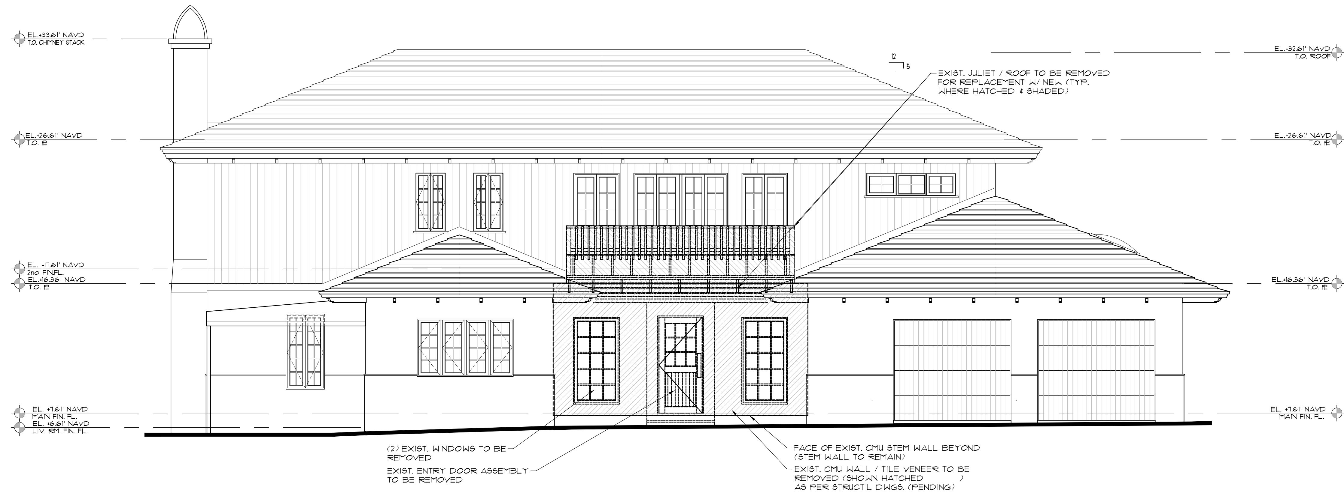
Proposed Demolition- Front (South) Elevation
