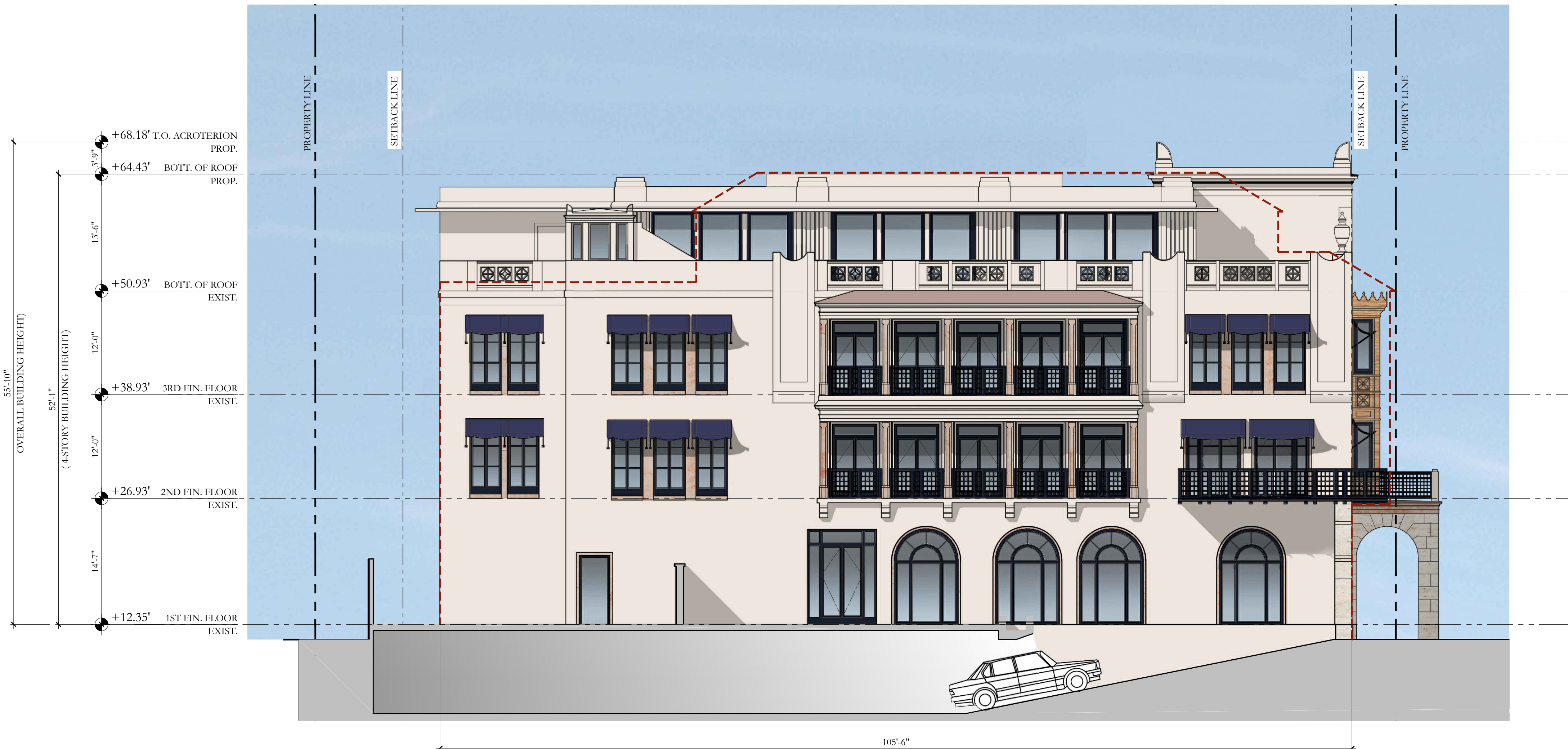
2 PROPOSED WEST ELEVATION 1/8"=1'-0"
