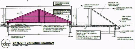
In all, the exterior changes are an overall improvement and will be minimally seen from the rightsof-way. The thirty feet x 30 feet skylight will be hidden from view by the existing 8'-6" high roof mansard roof structure.
