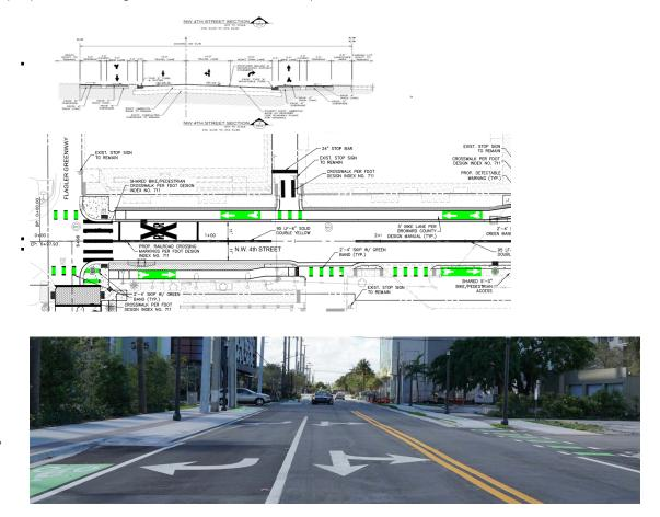
Flagler Greenway - "shared use path" with two way cycle track and sidewalk with pavement markings
