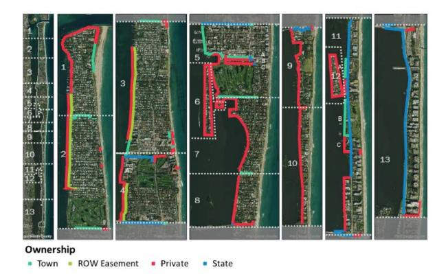
Figure 8 Potential neighborhood-scale flood control units and system alignments. These "flood control units" are not intended to align with the traditional Coastal Program shoreline "Reaches."
