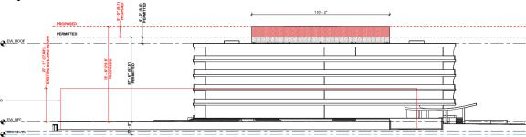
**Variance #10** is a variance to allow perimeter walls to exceed by 1'-0" for 6'-10" in front yard and 7'-6" in side yards. Walls located on these property lines must be measured from adjacent grade. Since the applicant is seeking to significantly raise the overall height of the parcel through adding fill to the sides and front and rear yards, the code maximum height does not work. The proposed variance request falls along the south property line and is shown below.
