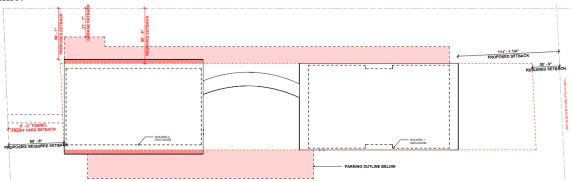
The other side setback variance to reduce the required minimum south side yard setback to 29'-2" in lieu of 62'-6". This distance is measured to the edge of the underground garage. However, it must be noted that the above grade structure (building 2) also does not comply—with a portion of the projecting balconies at all levels have a setback of 56'-1".
