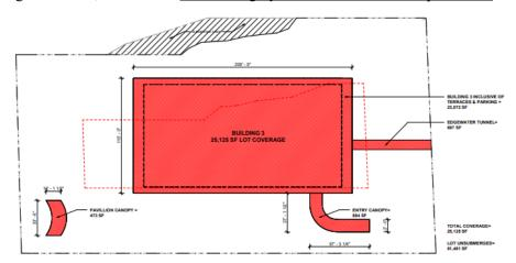
The underground garage level counts towards the lot coverage, including when it is outside of the building envelope. In this proposed projecting balconies in the above ground levels align with the outline of the garage. The garage level measures approximately 110'-0" wide and spans 199'-9" deep into the 398'-0" long site to accommodate 38 parking spaces: 6 in private garages, 28 more
