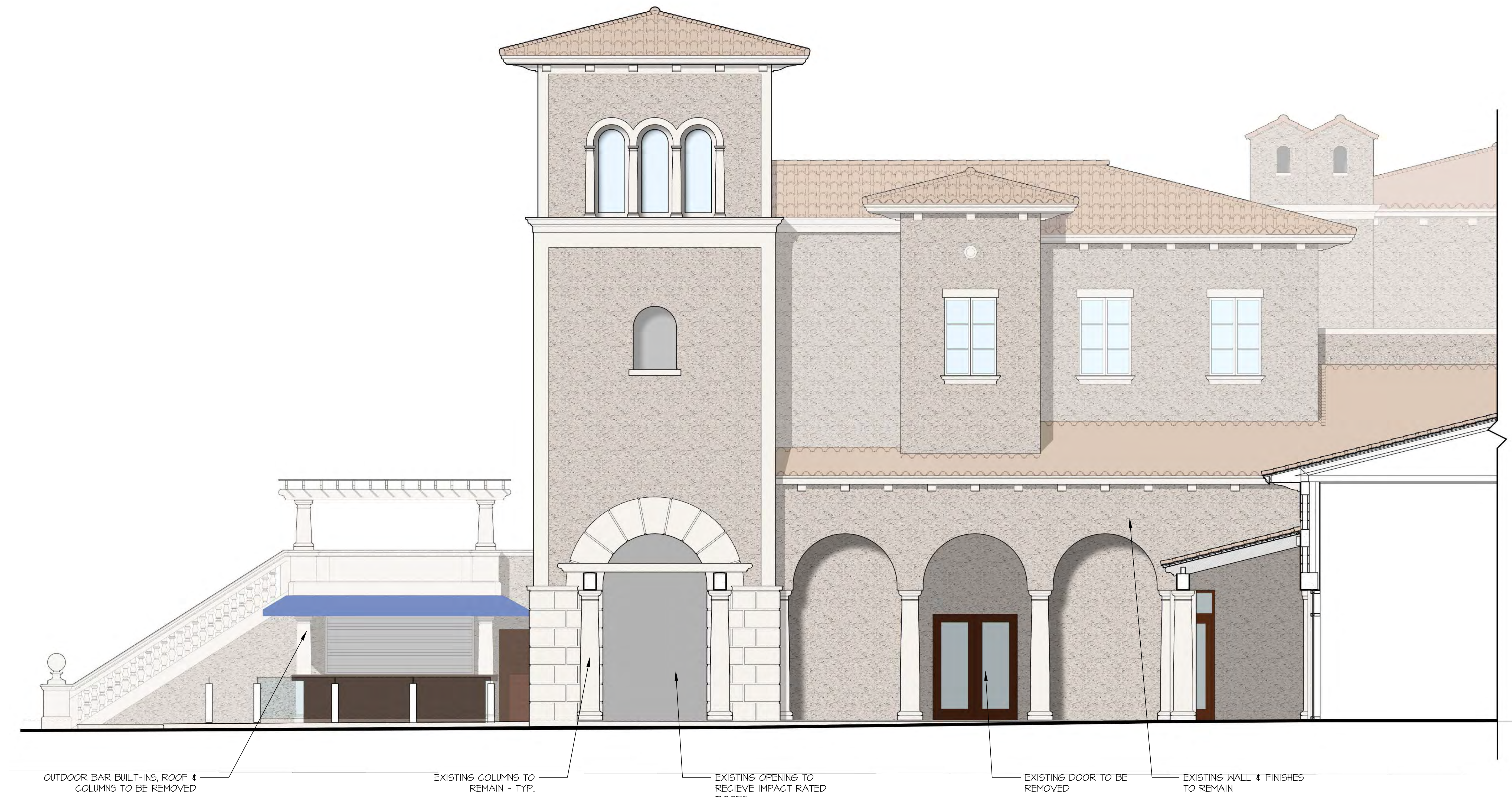
EXISTING NORTH ELEVATION
