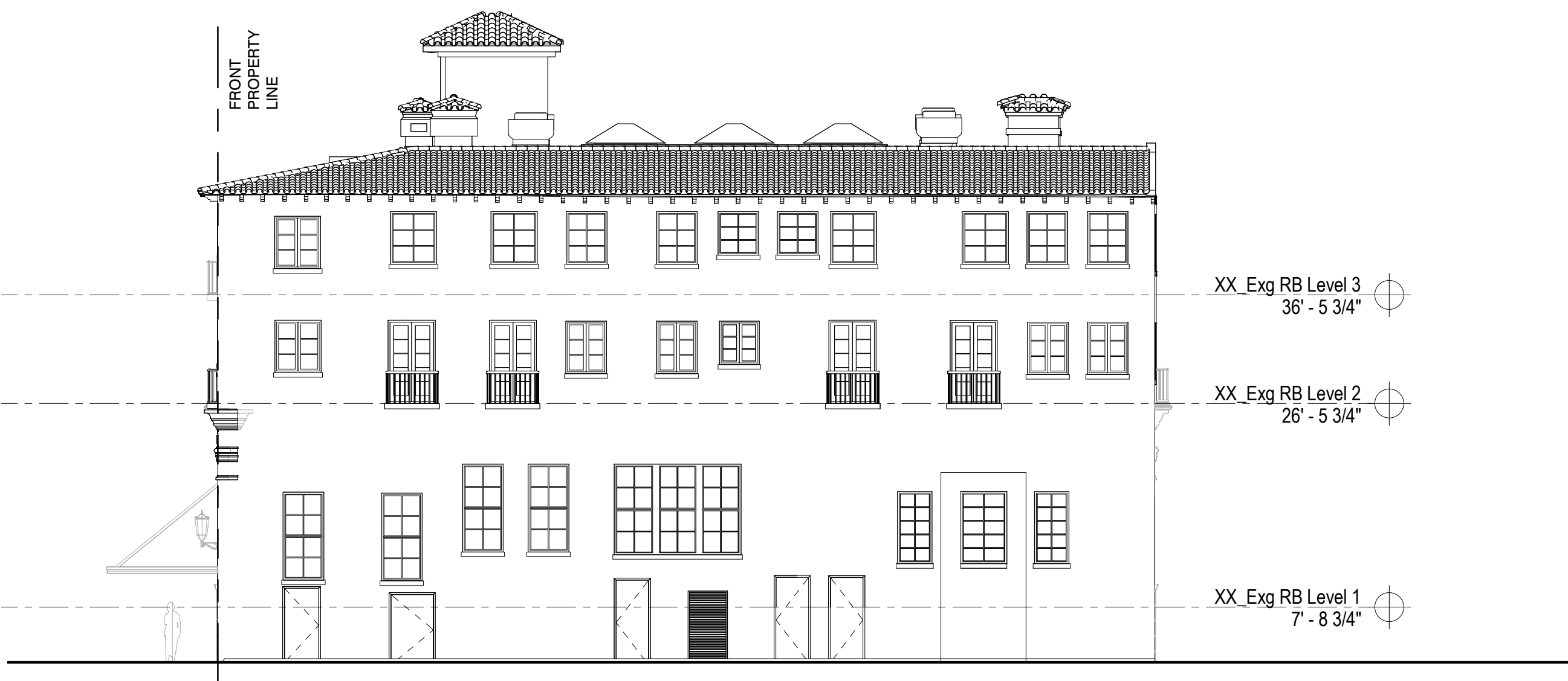
2 EXISTING NORTH ELEVATION (ROVENSKY BLDG) C-4.1.0 3/32" = 1'-0"
