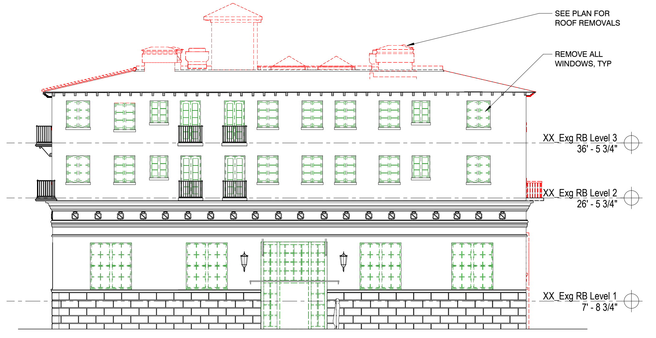
2 MATERIAL REMOVAL ELEVATION - EAST C-4.5.0 3/32" = 1'-0"
