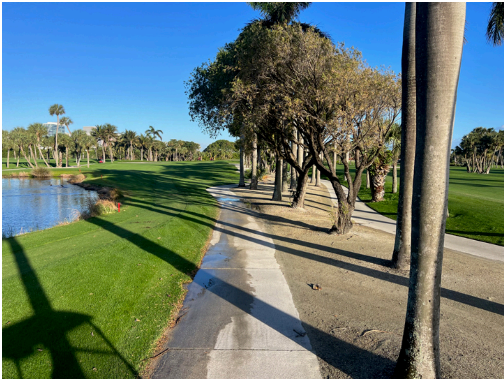
Low lying area on #6 tee during a dry weather pattern. Notice irrigation water is still standing on the cartpath. This interior area of the course will be raised significantly to prevent flooding after rains and during the king tide periods.
