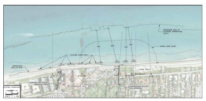
Figure 2: Breakwater Placement Location
