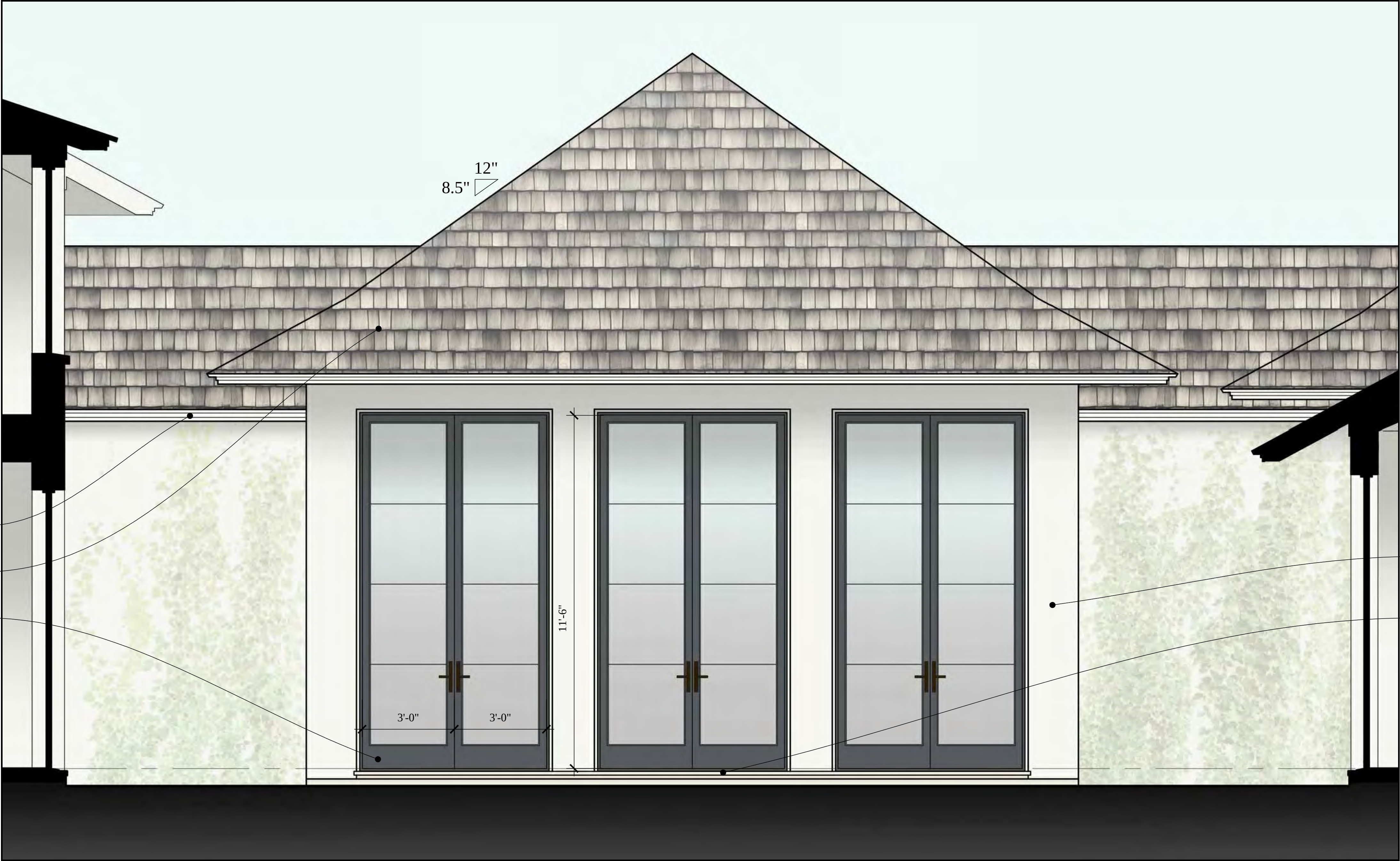
PARTIAL ELEVATION @ MAIN ENTRY
