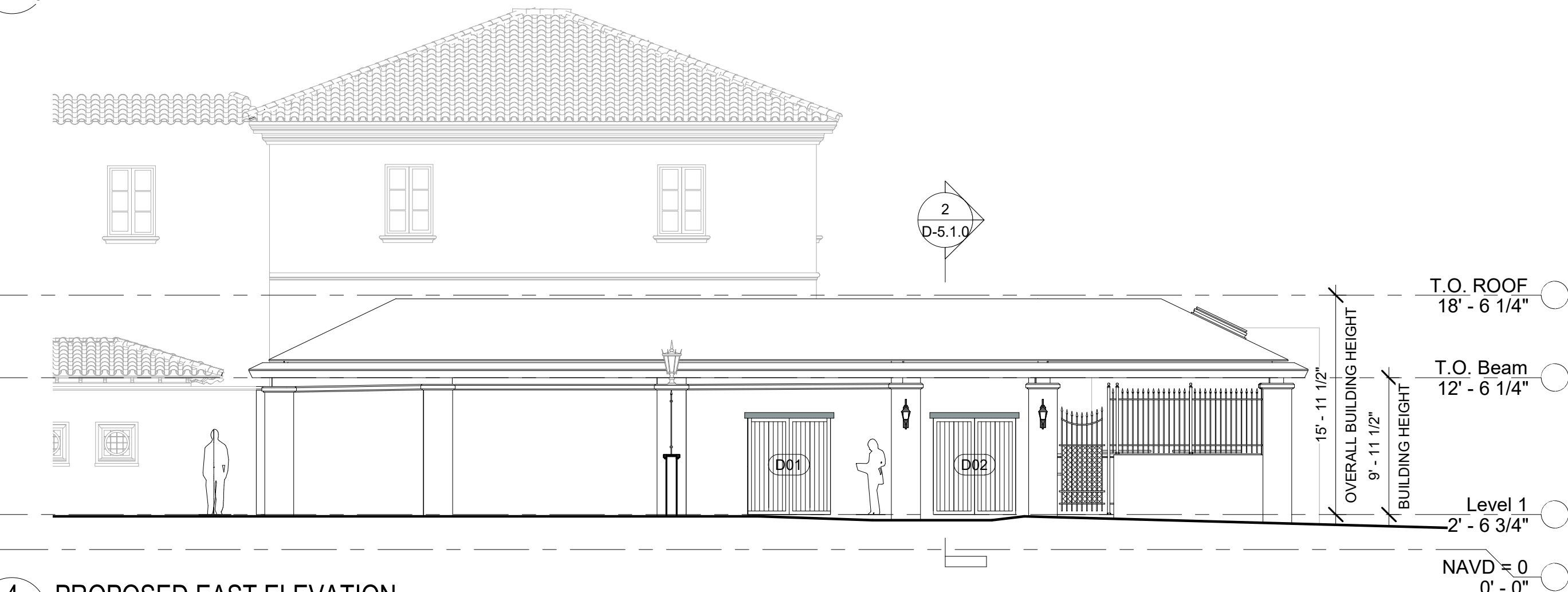
4 PROPOSED EAST ELEVATION D-4.1.0 1/8" = 1'-0"
