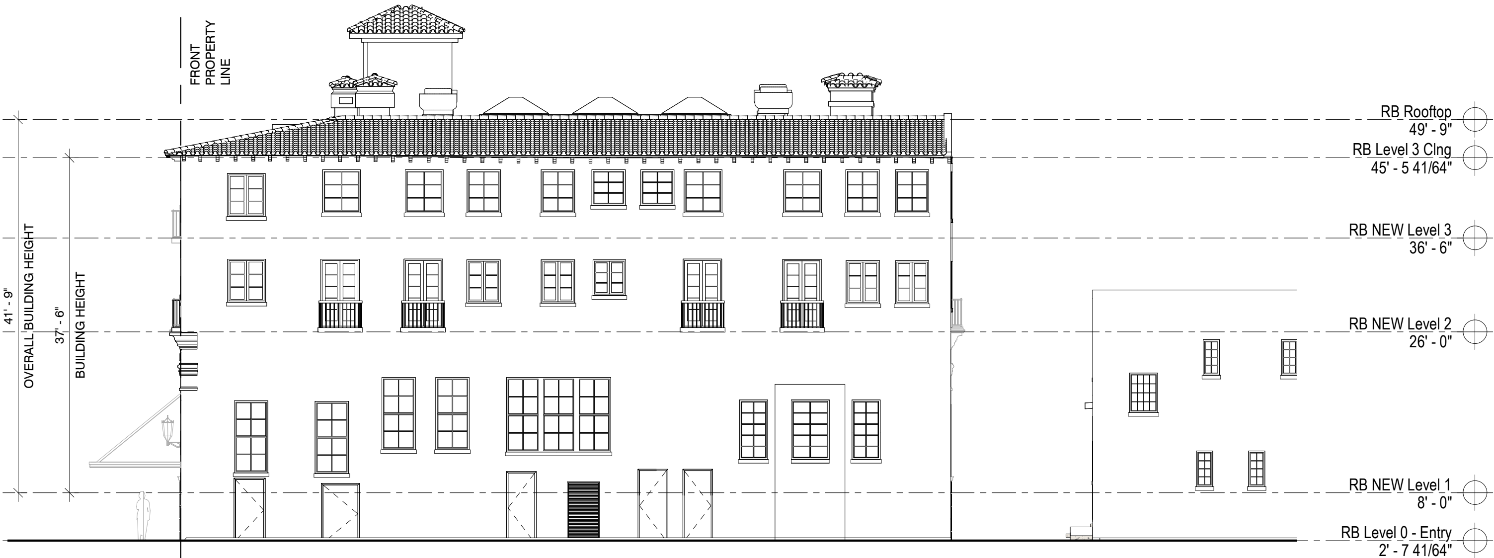
2 EXISTING NORTH ELEVATION (ROVENSKY BLDG) C-4.1.0 3/32" = 1'-0"
