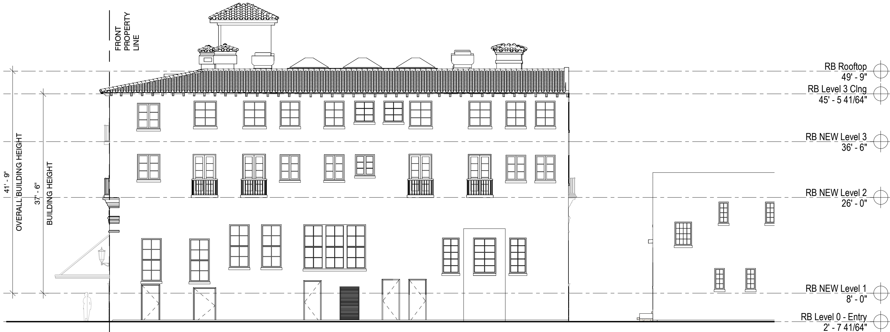
2 EXISTING NORTH ELEVATION (ROVENSKY BLDG) C-4.1.0 3/32" = 1'-0"
