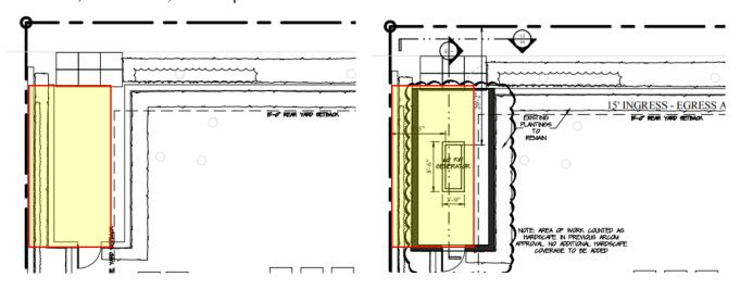
The subject parcel is very low, with a crown-of-road just under 3.41' NAVD. FEMA requirements mandate that new equipment be installed at minimum flood elevation, which is 7' NAVD. In doing so, the equipment must be physically raised off grade to the minimum requirement. Equipment located within yard areas are required to be screened by masonry walls as high as the equipment but are not permitted to exceed maximum wall heights. If the applicants chose to install a masonry
