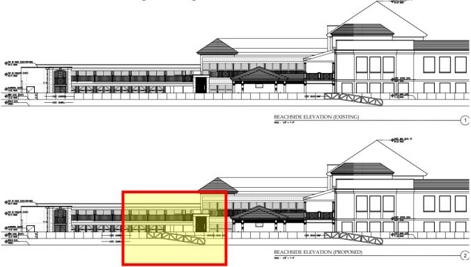
The proposed metal ramp will match the existing access ramp access ramp. It is proposed to be located at the southeastern edge of the property to provide additional ingress/egress from the pool deck for the members of the club, the total beach frontage is over 310' in length and a secondary means of access is greatly needed. The subject site is a Special Exception use in the R-B zoned 3.4 acre oceanfront site.
