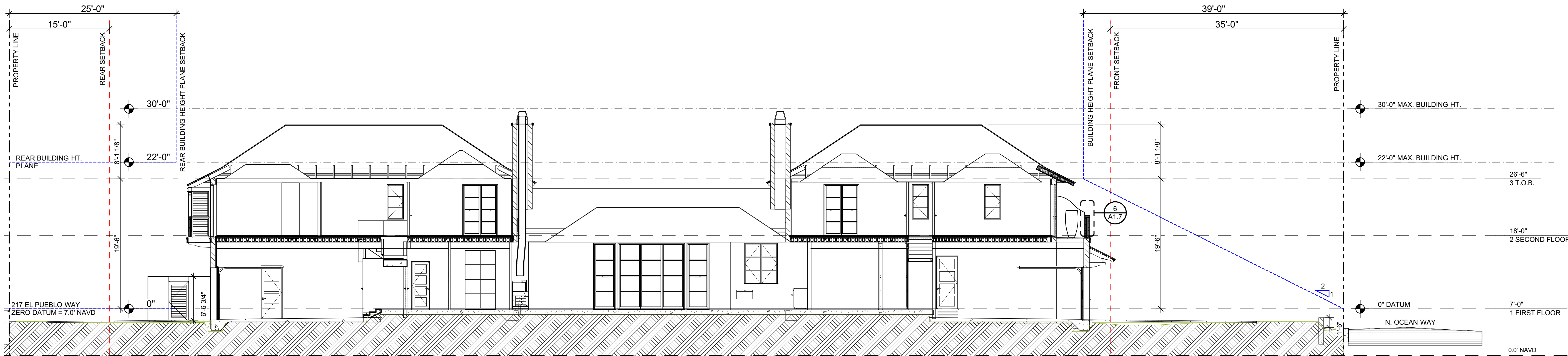
1 A1.6-1 PREVIOUSLY PROPOSED MAIN HOUSE SECTION AND HEIGHT PLANES SCALE: 1/8" = 1'-0"
