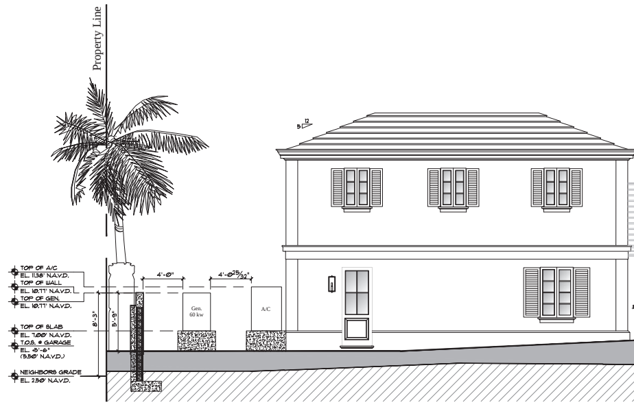
Proposed Equipment Enclosure Section @South Side
