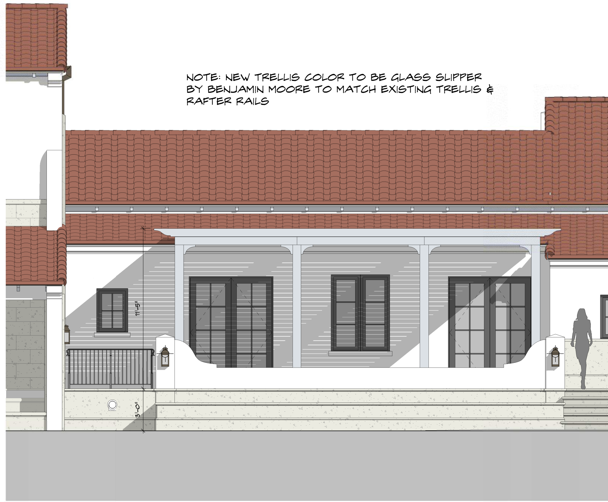
3 A2.0.1 TRELLIS - SOUTH ELEVATION - PROPOSED SCALE: 1/4" = 1'-0"
