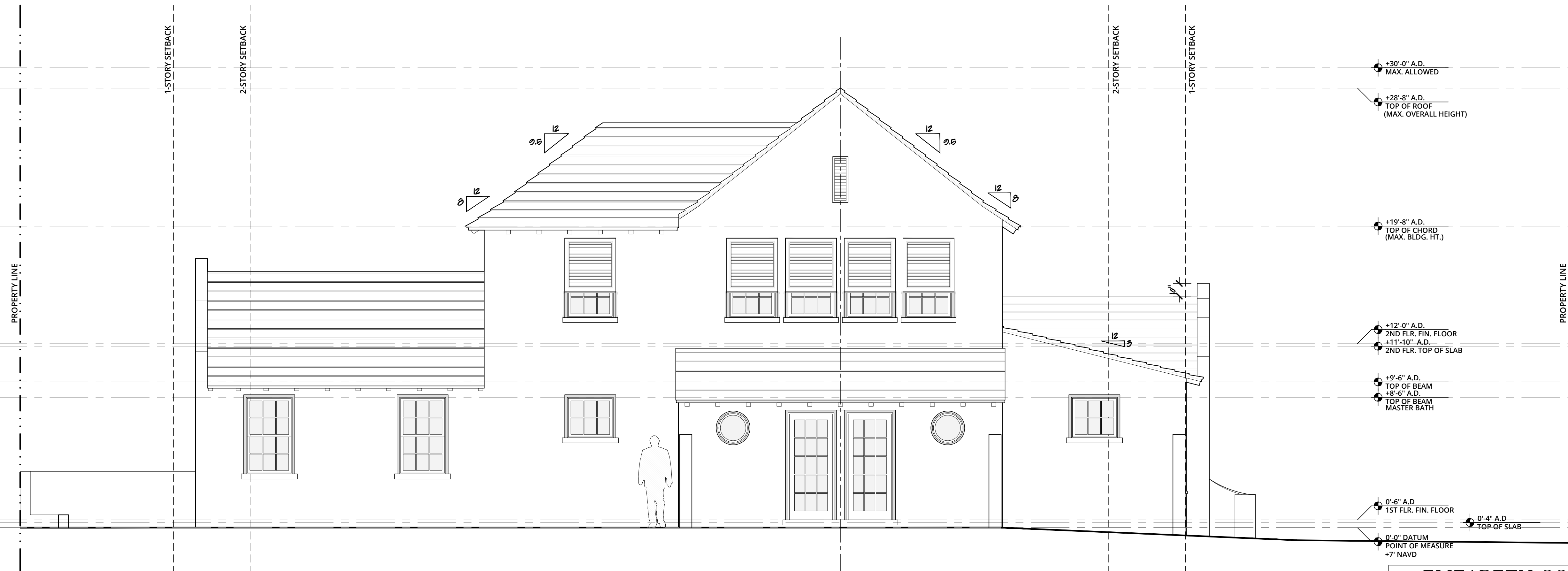
CURRENT EAST ELEVATION 1/4" = 1'-0"
