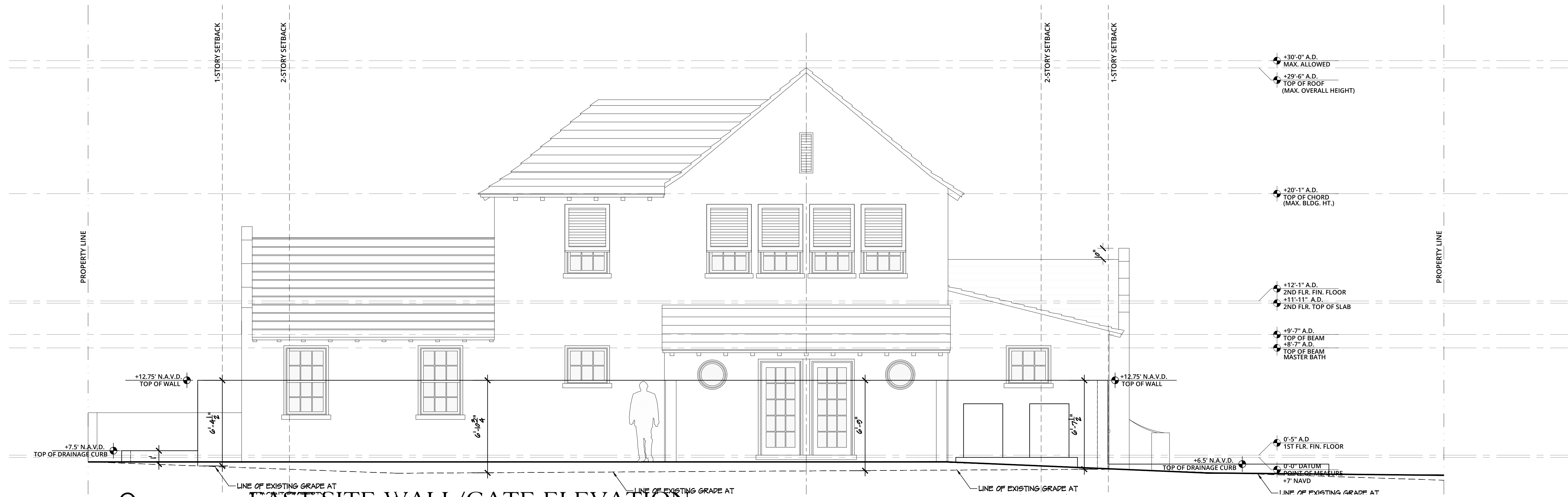
EAST SITE WALL/GATE ELEVATION SCALE: 1/4"=1'-0"
