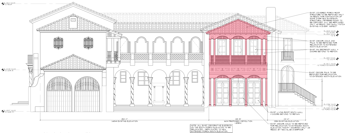
Proposed South Elevation Demolition Scale
