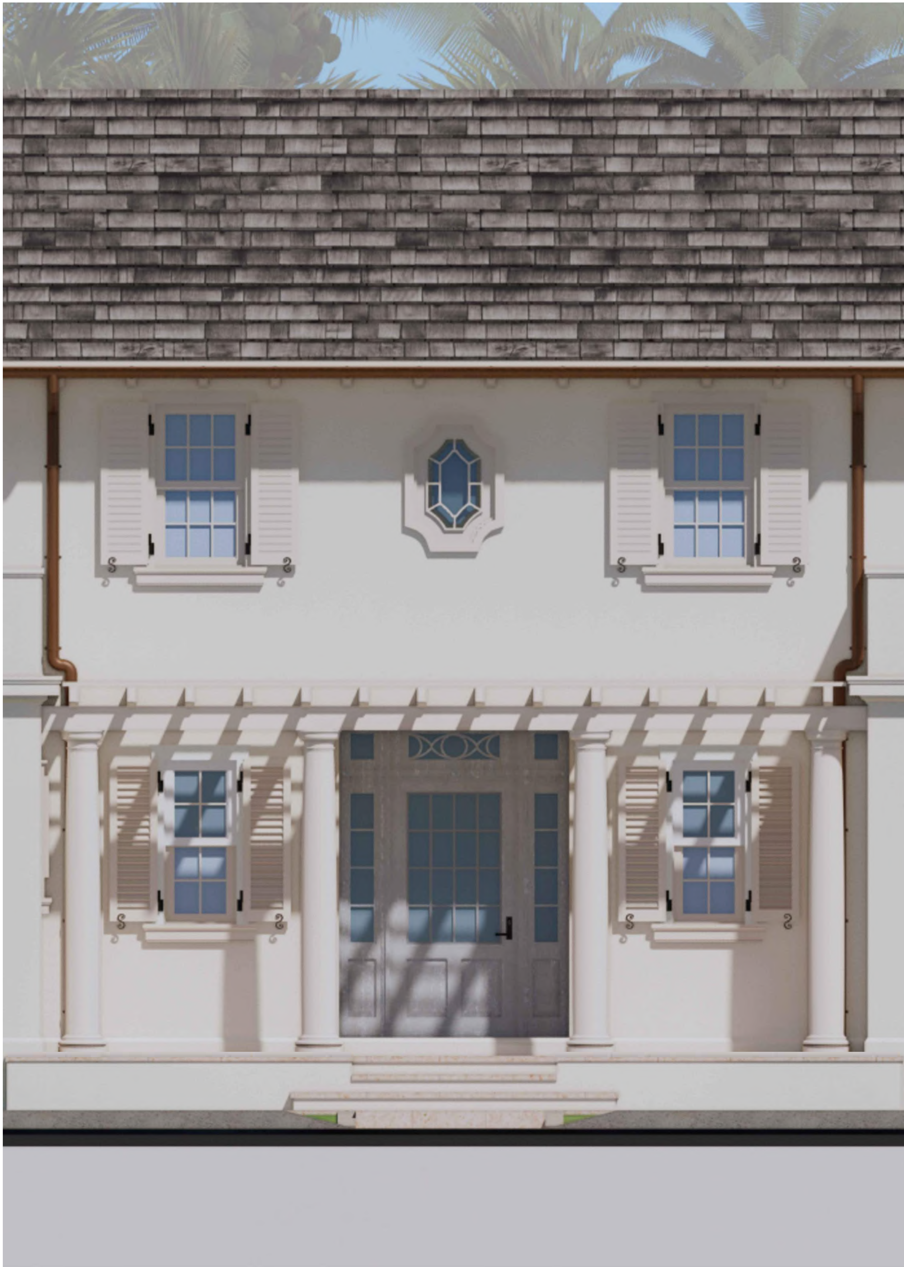
PARTIAL ENTRY ELEVATION N.T.S. COVERED ENTRY/PERGOLA
