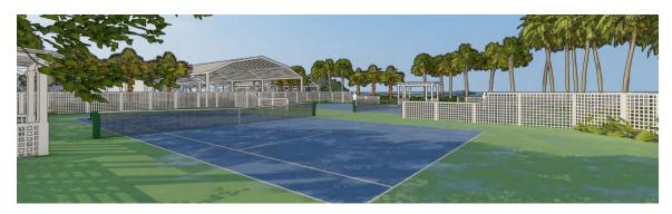
The fencing material is proposed to contain a white finish and the material is a synthetic composite product that the manufacturer (Walpole) describes as "Solid Cellular Vinyl." The white fencing has black coated wire mesh at all courts except for west side of center court and east court along
