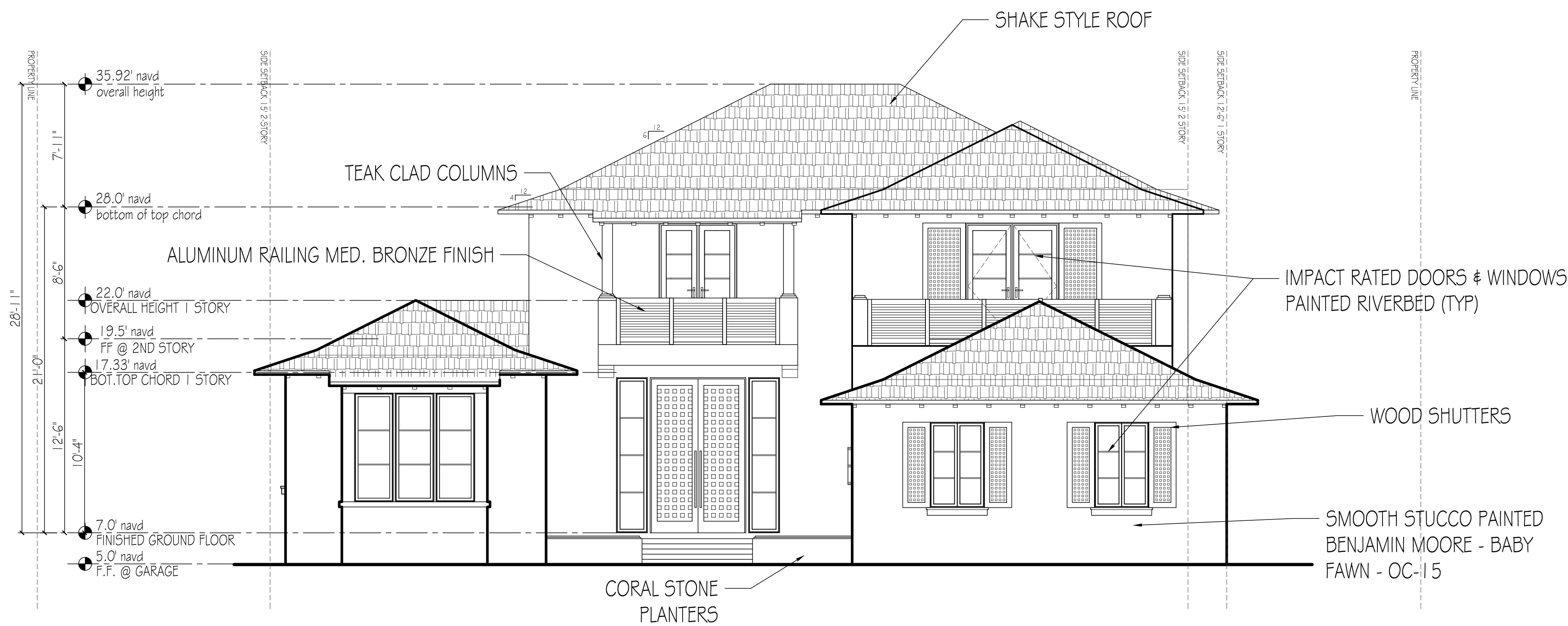
1 PROPOSED EAST ELEVATION 1/4" = 1'-0"
