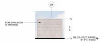
2 SECURITY BUILDING 2 - SOUTH ELEVATION A.35 SCALE: 1/8" = 1'-0"
